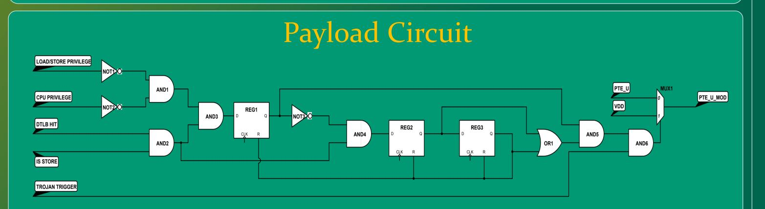
The payload circuit targets Ariane's Memory Management Unit (MMU). Payload circuit design has a minimal footprint, as it requires only 14 logic gates.
