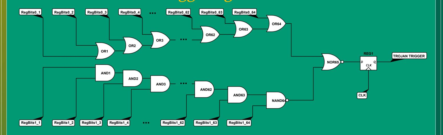
The trigger circuit targets Ariane's General-Purpose Registers (GPRs), as it monitors them for specific byte values to assert the trigger signal. Triggering circuit's design is scalable. For the worst-case scenario of a 128-bit magic value, it requires only 130 logic gates.
